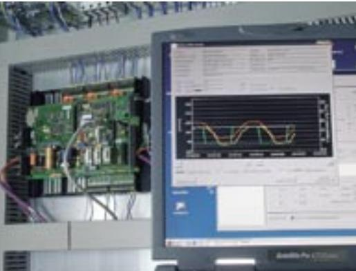
The Belimo PC-Tool allows volumetric flows and trend records to be graphically displayed on a laptop and fault diagnostics and corrections to be performed in an easy way – either from the control cabinet or directly on site with the device.
